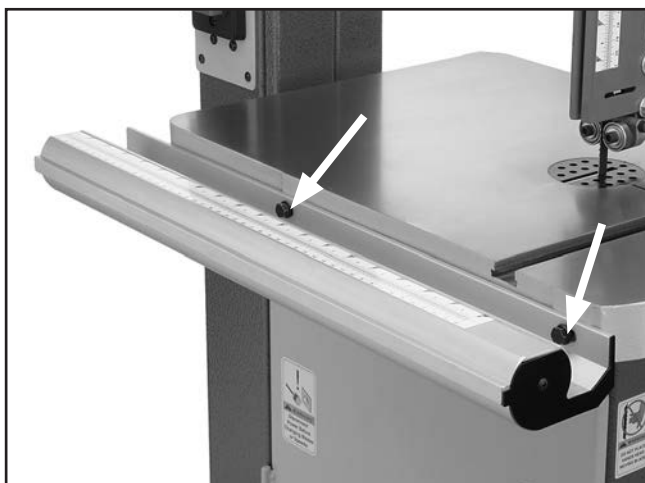
Figure 17. Installed front rail.
